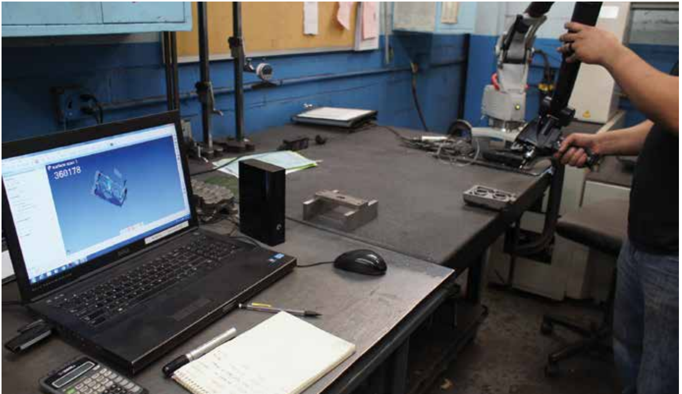
An employee checks the dimensions of a casting to the CAD file specifications in Osco Industries quality control lab.
